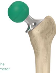
To prevent destruction of the press-fit mechanism, the dimension of stem trial is reduced by 0.2 mm in diameter when compared with the size matched broach. As shown below, the U2 revision hip instrumentation design provides a 0.5 mm interference between the real implant and the broach to enable stable initial fixation.
